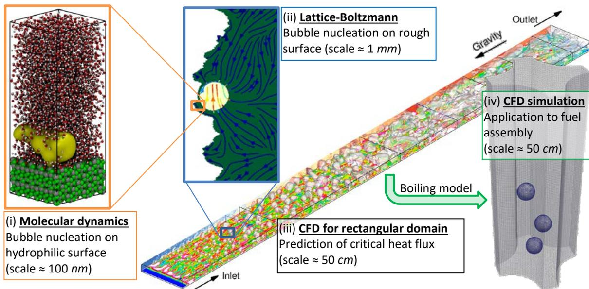
Fig. 1: Simulation system for the prediction of Critical Heat Flux (CHF) in a fuel assembly.
