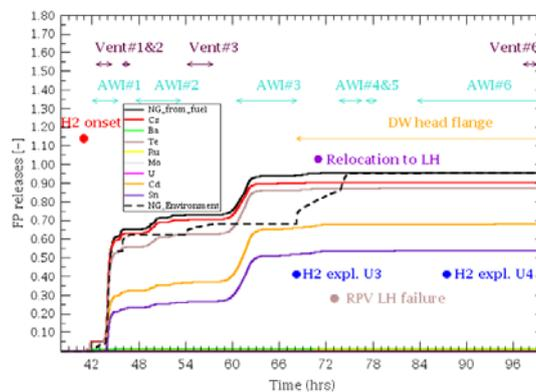
Fig. 3: Fission product release from the fuel and noble gas release to the environment in the reference sequence
